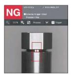
(Component assembly misalignment check)
