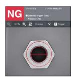
(Diameter-based difference check of metal components)
